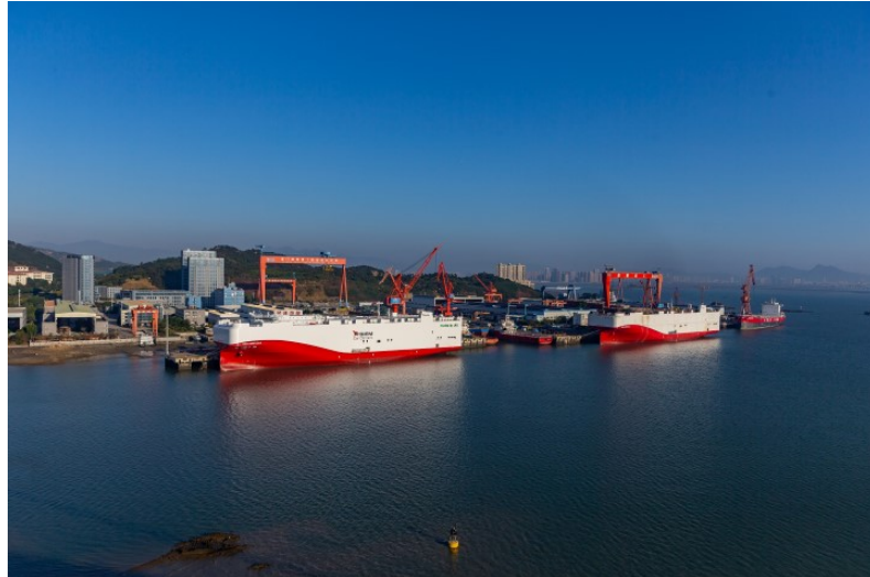
The 'Siem Confucius' and sister ship, the 'Siem Aristotle', are the very first trans-Atlantic PCTCs (Pure Car Truck Carriers) to operate full-time on LNG
