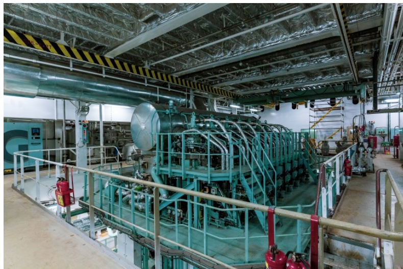
Both vessels have MAN B&W S60ME-GI (-Gas Injection) dual-fuel, two-stroke main engines that each deliver 12,600 kW with direct injection and exhaust-gas treatment to further reduce emissions
